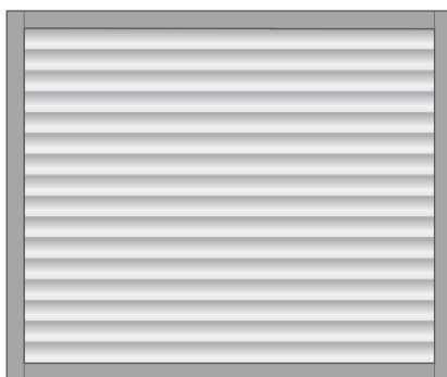
Infill Designs No 8 to 11- Horizontal Louvre Infill No 8 - 58mm Louvre, No 9 - 80mm Louvre No 10 - 120mm Louvre, No 11 - 150mm Louvre
